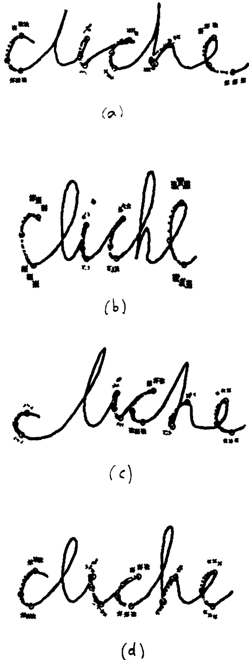
Fig. 8. Compensating for handwritten shape variability by an affine transform (see text). Here, the system looked for instances of the c -like stroke in four examples of the word cliche , written by four different subjects. The detected instances are marked by the dotted lines. The shaded areas correspond to the "forbidden" regions (see figure 7). Note that there is no objective way to determine whether a c -like stroke should be found in the input. It is easy to see, however, that out of the entire variety of c -like strokes that seem to be present in these images (20 instances) only one was missed (the borderline case that is a part of the h in (b)). The control points in the image were detected automatically in all cases.
